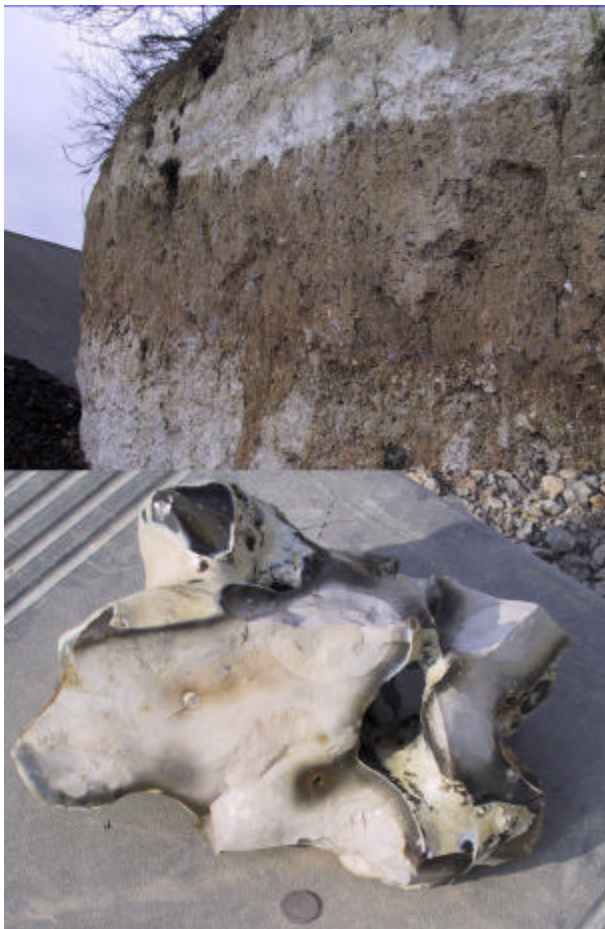
Fig. 2 Above: Rock Section Showing Chalk Strata Below: Flint Nodule with 20 pence for scale
